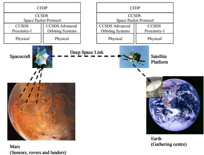
Fig. 1. Reference Scenario and CCSDS Protocol Stack
