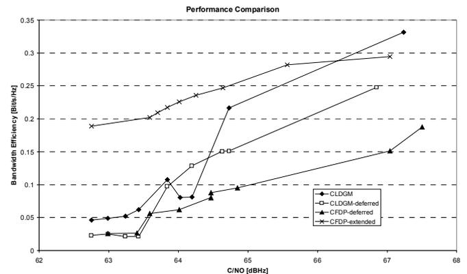
Fig. 7. Performance comparison: Bandwidth Efficiency vs  $C/N_0$
