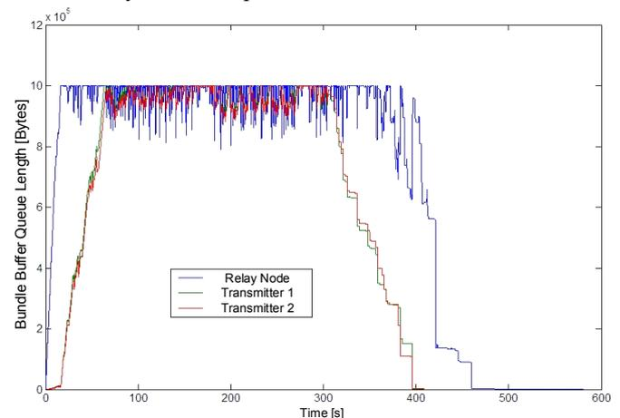
Fig. 4. Bundle Buffer Queue Length in case of 1 Mbytes buffer capacity (all DTN nodes) and propagation delay 5 s.
