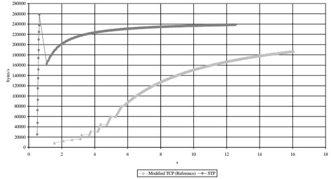
Fig. 7. Throughput versus time, 3 Mbytes, mono-connection.
