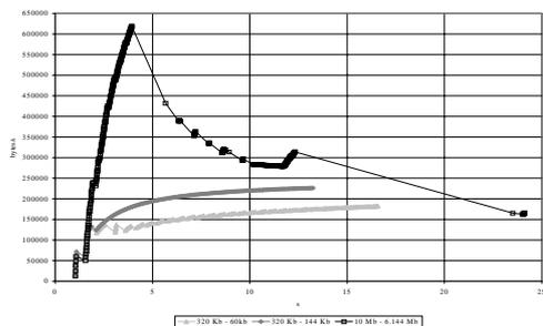
Fig. 4. Throughput vs time, 3 Mbytes, K=10, IW=6, IP-TCP buf.
