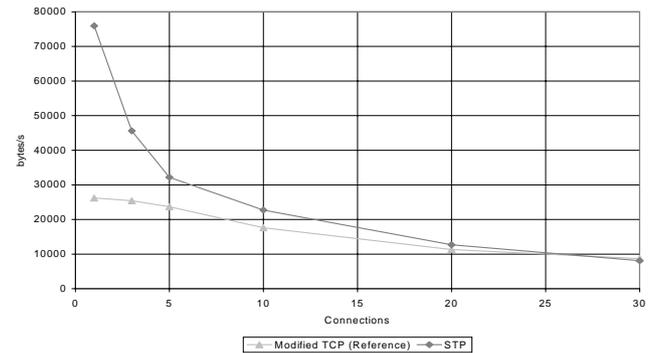
Fig. 9. Throughput versus number of connections, 100 Kbytes, multi-connection.
