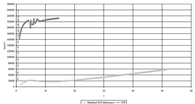
Fig. 10. Throughput versus time, 3 Mbytes, mono-connection, packet loss.
