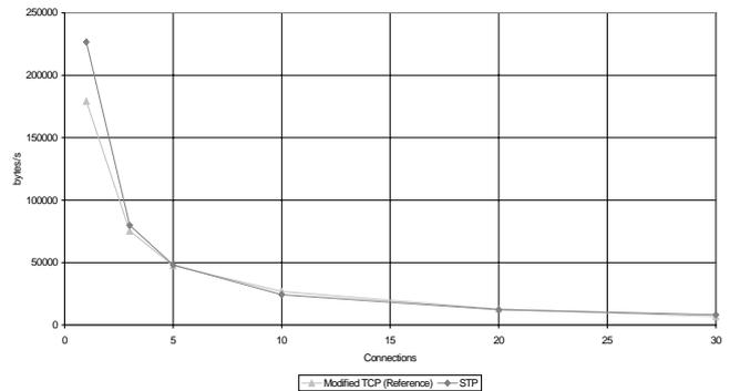
Fig. 8. Throughput versus number of connections, 3 Mbytes, multi-connection.
