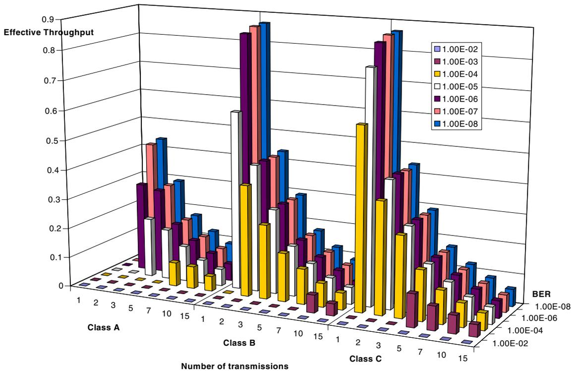
Fig. 8. Effective Throughput for different traffic classes, CFDP-UE-RT.
