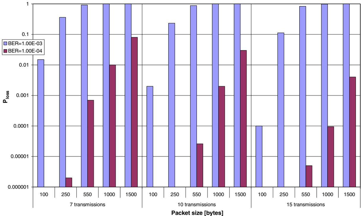
Fig. 7.  $P_{\text{loss}}$ , 7, 10 and 15 transmissions, CFDP-UE-RT.
