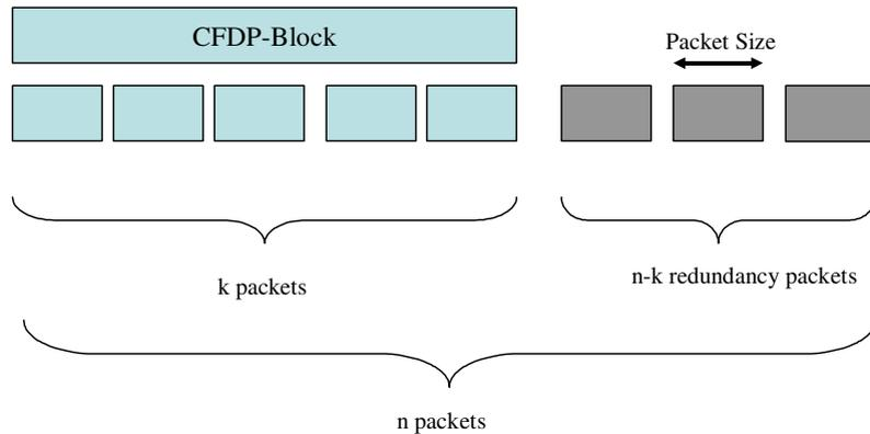
Fig. 1. CFDP-UE-RSE Creation of Redundancy Packets.
