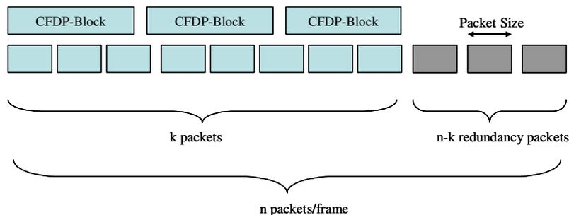
Fig. 2. CFDP-UE-LDPC Creation of Redundancy Packets.
