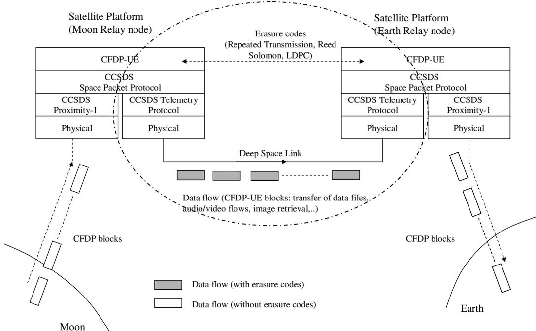
Fig. 4. The testbed and the CCSDS protocol architecture.
