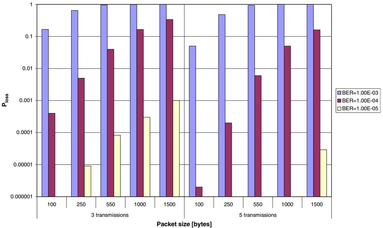
Fig. 6.  $P_{loss}$ , 3 and 5 transmissions, CFDP-UE-RT.
